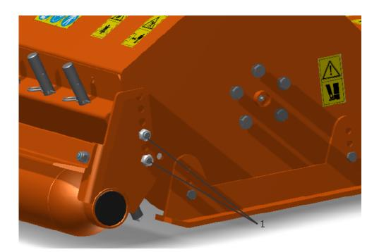
Depending on the different roller positions, it is possible to set four different cutting heights: 32-57-82 and 107 mm.
