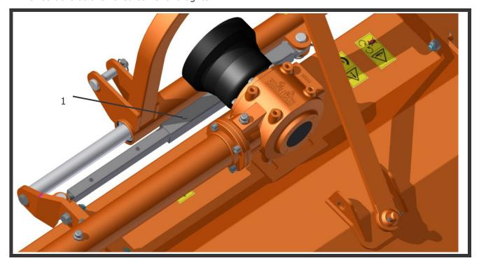
In case of configuration with hydraulic cylinder, the side adjustment of the frame is effected by actuating the cylinder directly by the hydraulic control system of the tractor, after performed the connection of the machine hydraulics to the tractor.
