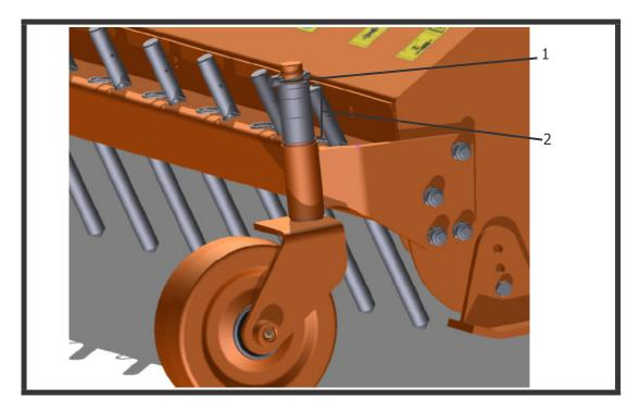
Depending on the different position of the spacers on the shaft, it is possible to set five different cutting heights: 70-76-89-114 and 145 mm.
